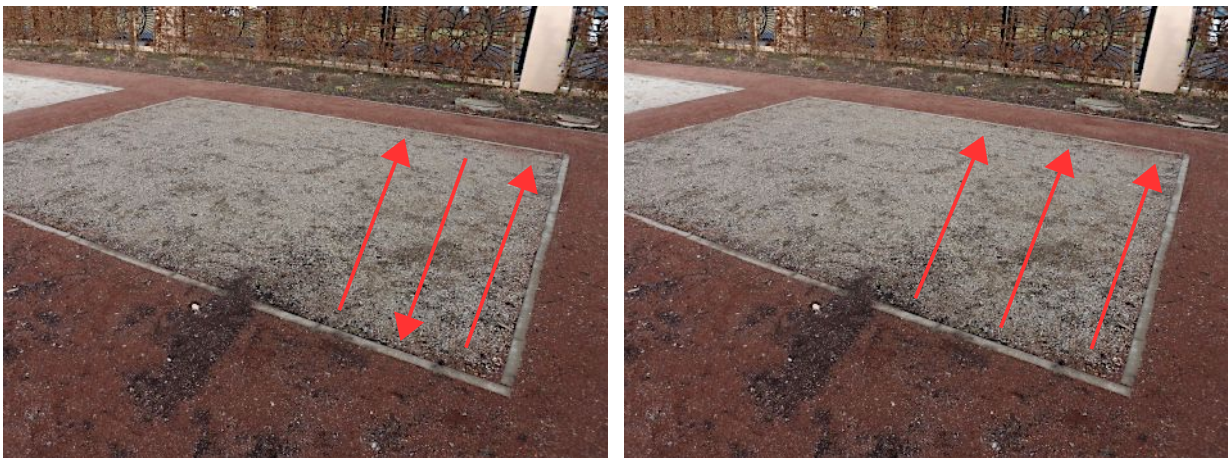
Figure 7.3: "Zig-Zag" scanning (left) and "Parallel" scanning (right)
