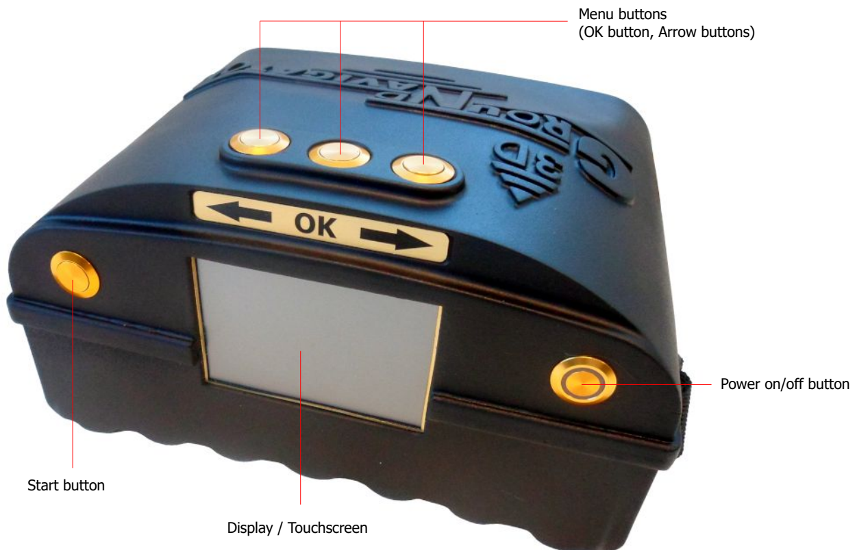
Figure 5.2: Control elements of the top and front panel
