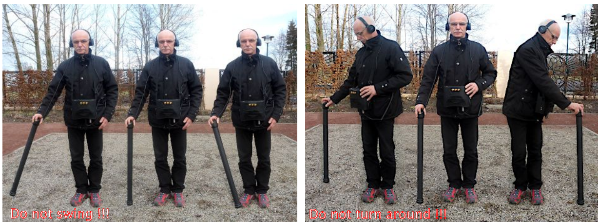
Figure 7.10: Pivoting or turning the probe falsifies the measurement
